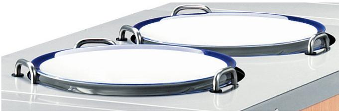
Adjust the guide bars for the plates for the required plate size. Check that the adjusting pivot in the end of each guide bar is in the same place. Note a non-central plate load could damage the plate elevator and weaken its operation.
