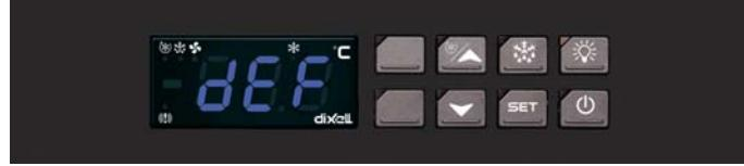
**Note!** The manual defrosting resets the defrosting time counter so that by means of the manual defrosting period the regular defrosting periods can be scheduled to take place e.g. outside the peak periods.
