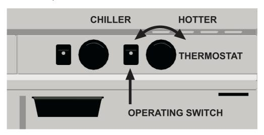
Switch on the operating switch. The signal lamp will indicate the start-up, and the resistors will switch on.
