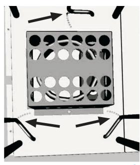
Non-central plate load may damage the dispenser and cause malfunction.
