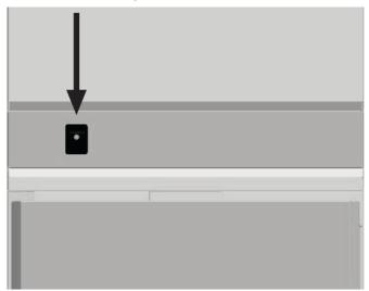
The thermostat knob is located inside the front plate cylinder.
