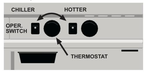
Switch on the operating switch. The signal lamp will indicate the start-up, and the resistors will switch on.
