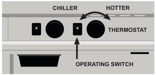
Switch on the operating switch. The signal lamp will indicate the start-up, and the resistors will switch on. Regulate the water temperature by the thermostat.
