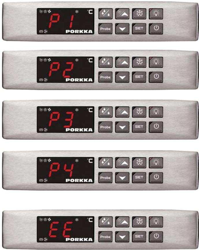
**"P1"**      Thermostat probe failure\*\*\*
