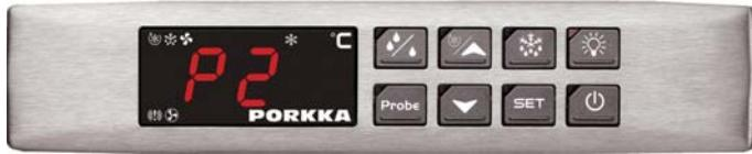
**"P2"** **Evaporatorgivare defekt\*\*\*
