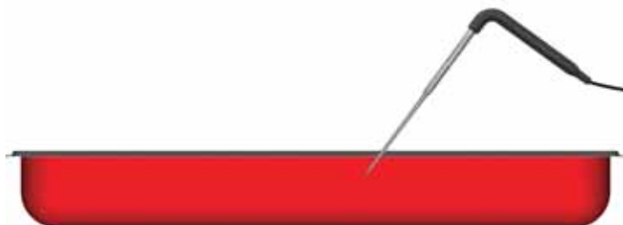
2B. Place the probe closer to surface when chilling food staffs that are more likely to freeze easily.
