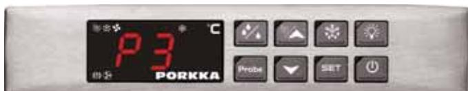
"P3" Condenser probe failure\*
