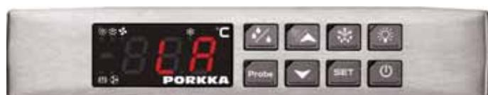
Reset the alarm signal by pressing any button.
