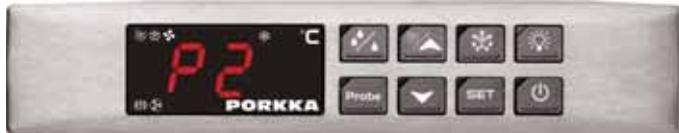
"P2" Evaporator probe failure\*
